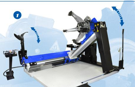
Tools holding arm and clamping chuck arm move in synch, keeping the tools perfectly tangent to the wheel, thus reducing tension and protecting rim and tyre from any damage.
