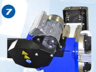
Clamping chuck is powered by a 3 speed motoinverter, including low speed for tyre tread sculpting:
